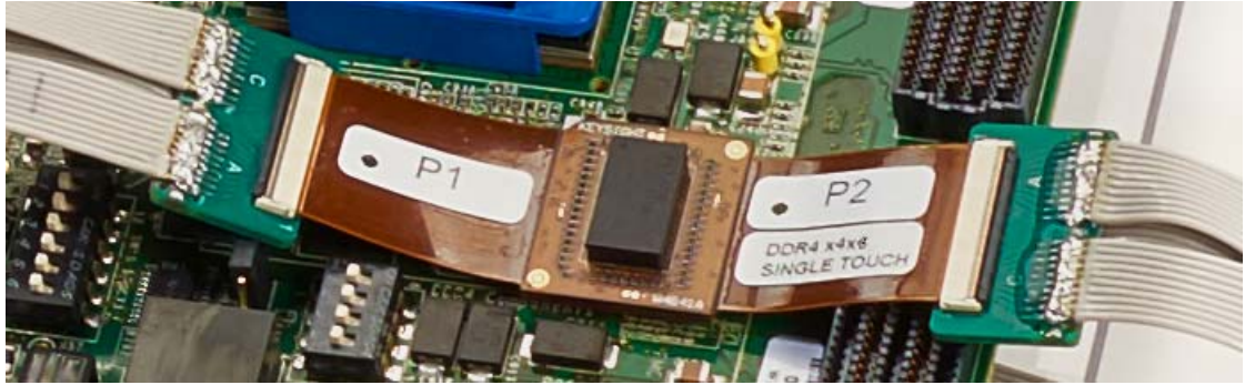
Figure 42 W4643A interposer attached to U4208A and U4209A ZIF connectors
