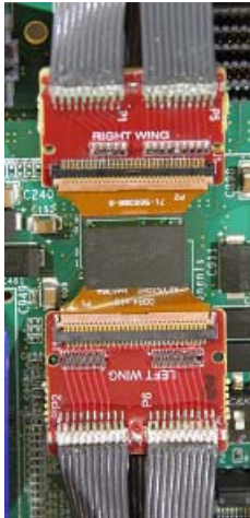
Figure 38 W4636A interposer attached to E5847A ZIF connectors
