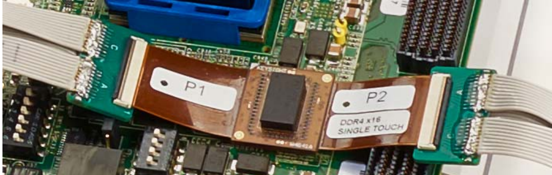
Figure 46 W4641A interposer attached to U4208A and U4209A ZIF connectors
